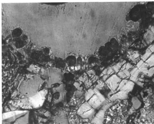
Figure 21. Amorphous iron-manganese oxides lining wall of an empty vesicle. Sample 424C-2-1 (Piece 7). Transmitted light; \times 16 .
