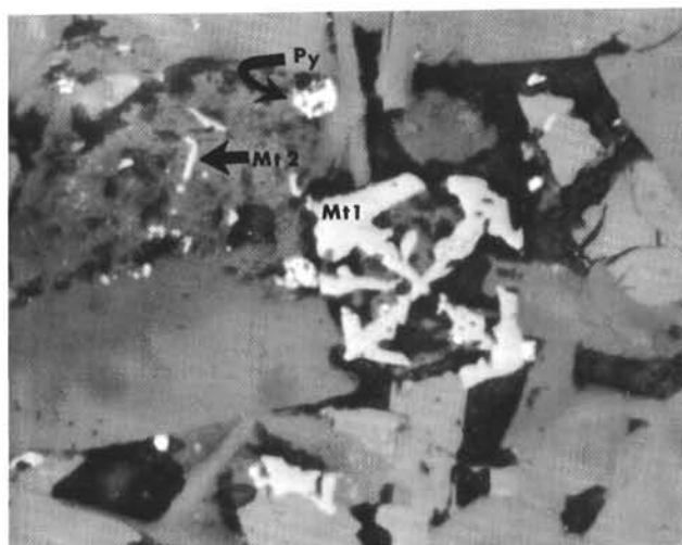
Figure 17. Skeletal Ti-magnetite in interstitial glass. Also sulfide spheres and second-generation Ti-magnetite in glass. Sample 428-5-4, 15-18 cm, reflected and transmitted light; \times 16 . Mt1 = first generation Ti-magnetites; Py = Py sphere; Mt2 = second generation Ti-magnetite.
