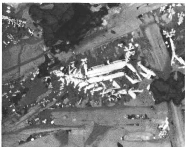
Figure 5. Rectilinear arrangement of skeletal Ti-magnetite crystals. Sample 424-5-1, 31–34 cm; reflected light; \times 16 .
