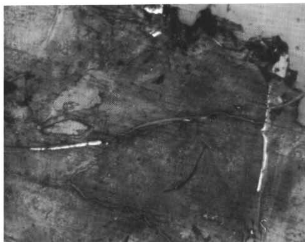
Figure 18. Silicate glass, altered to smectite, veined by pyrite. Sample 428A-5-3, 123-126 cm; reflected and transmitted light, \times 16 .
