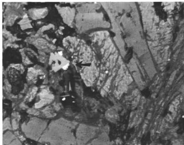
Figure 9. Pyrite spheres flattened against subhedral Ti-magnetite. Both opaque phases occur in interstitial glass. Sample 424-4-6, 112-116 cm; reflected light; \times 16 .
