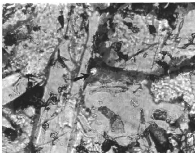
Figure 4. Pyrite sphere in glass interstitial to feldspar laths. Sample 422-7-1 (Piece 11); reflected and transmitted light; \times 16 .
