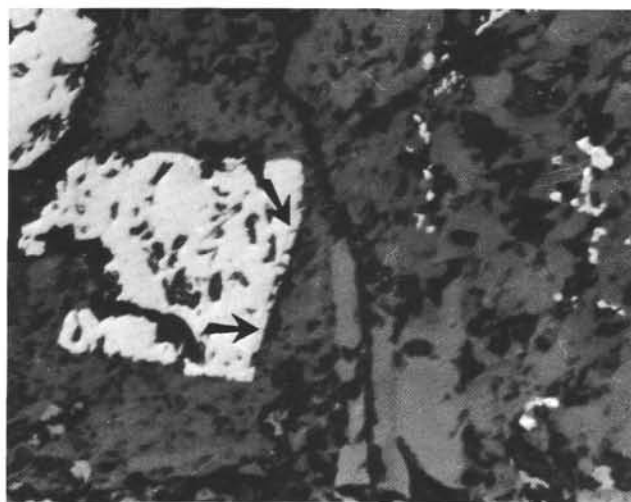
Figure 7. Subhedral Ti-magnetite with pyrite rim (indicated by arrows). Sample 424-2-6, 112–116 cm; reflected light; \times 16 .
